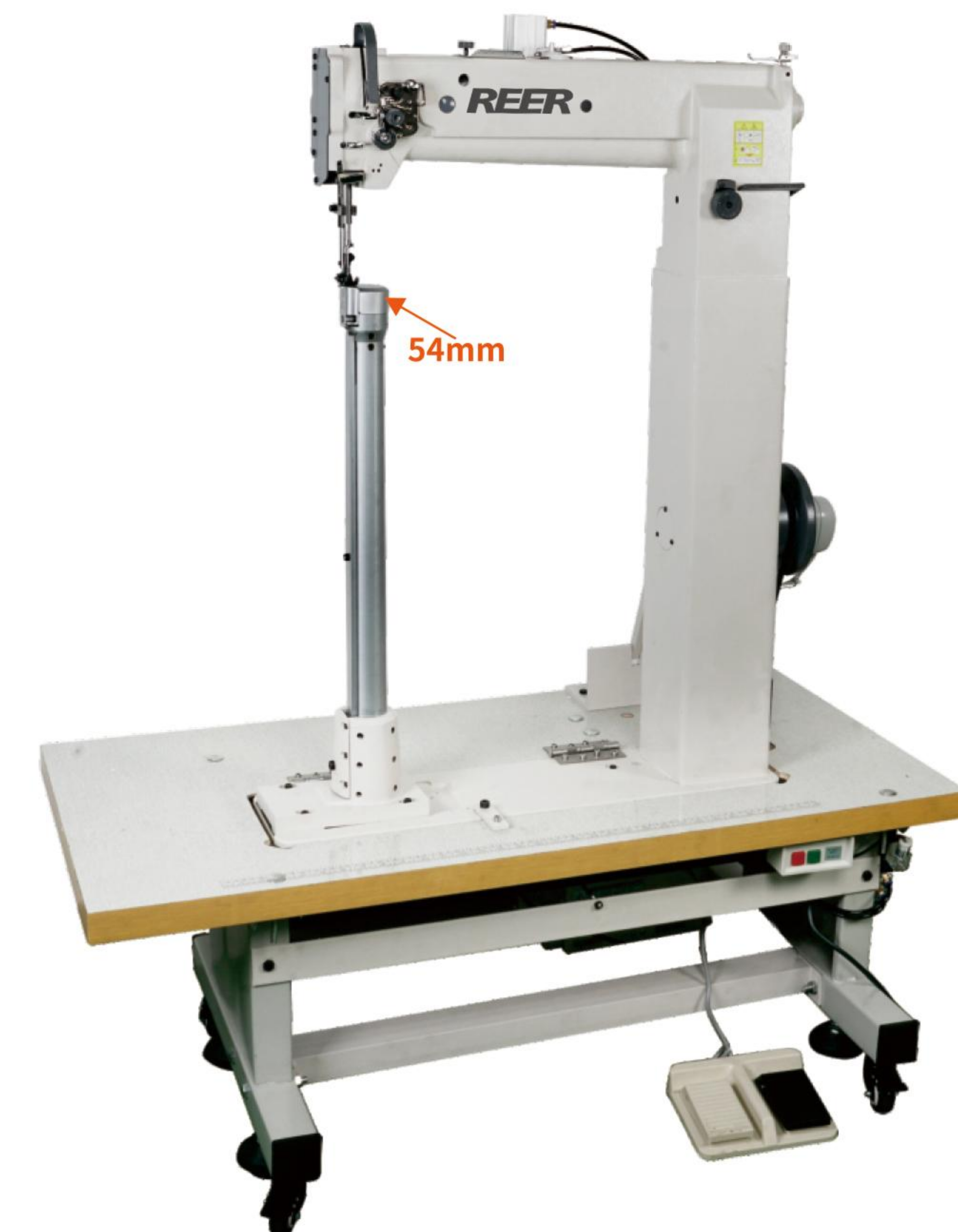
R8918-15/R8918-18 竖筒型综合送料高柱车 Post Bed Walking Foot Lockstitch Sewing Machine
