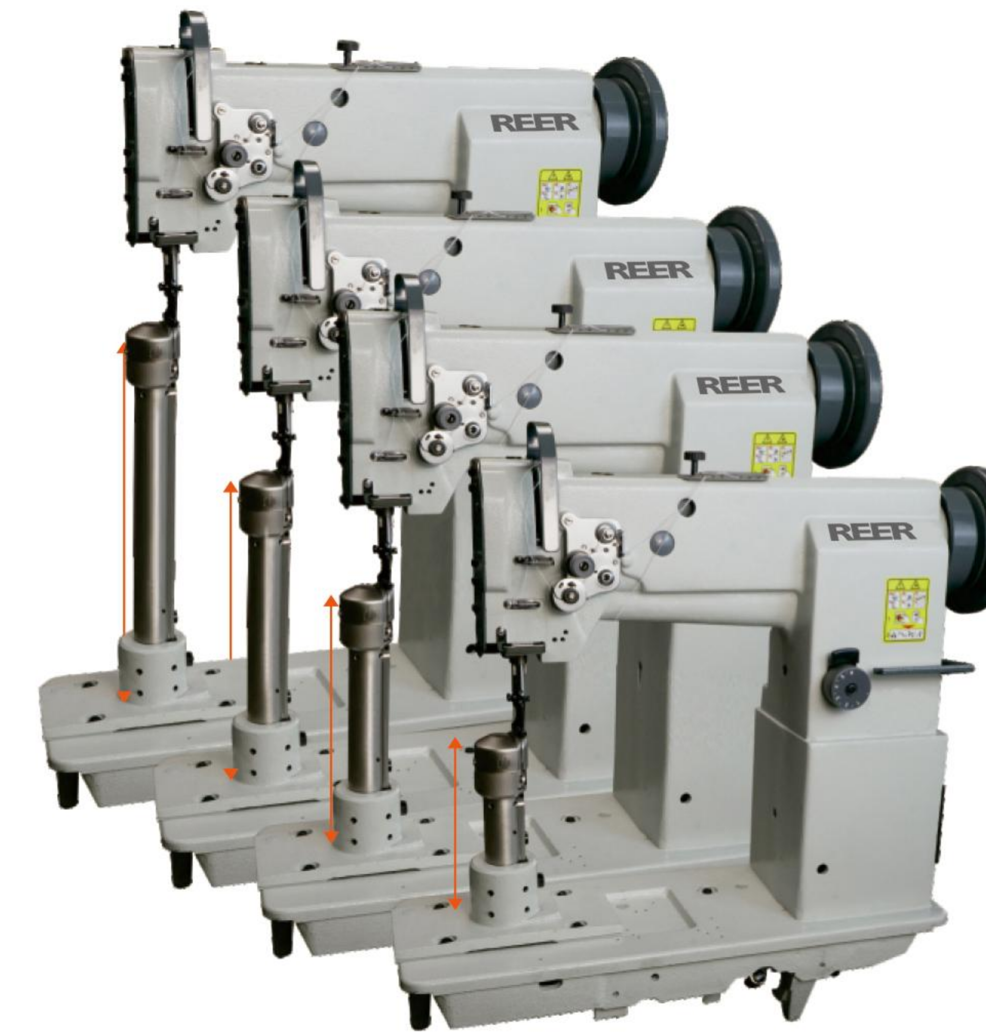
柱高可选尺寸180/250/305/350mm Post height optional size: 180/250/305/350mm
